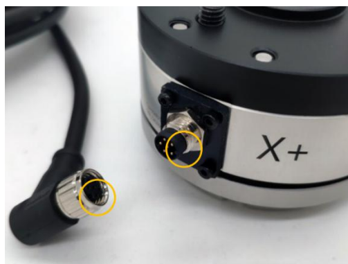
Cable Connection Operation
