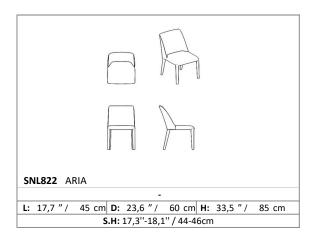
Inner StructureBackSittingLegsMetal inner structureD32 foamHR35 foamSolid legs and fabric<br/>coated legs are used
