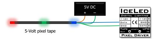
Note that the two ground wires should join at the tape not at the driver or supply.
