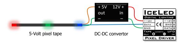
A common ground connection must exist between the 12V input and 5V output – if not a wire should link connect the two – (minus) terminals together.
