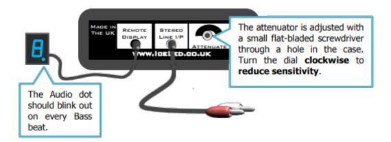
A direct line-level connection can be made to In Car Entertainment systems using a standard 3.5mm Stereo jack audio lead. This automatically disables the internal microphone so ensuring that music alone activates the light. The attenuator is still effective when a direct connection is used.
