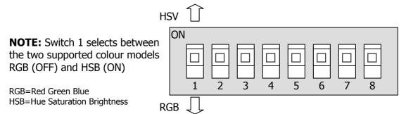
Switches 2 to 8 select between 128 different DMX base addresses in multiples of 4. To calculate the appropriate switch settings for a given channel note that each switch provides the following weightings **when moved to the ON position**:
