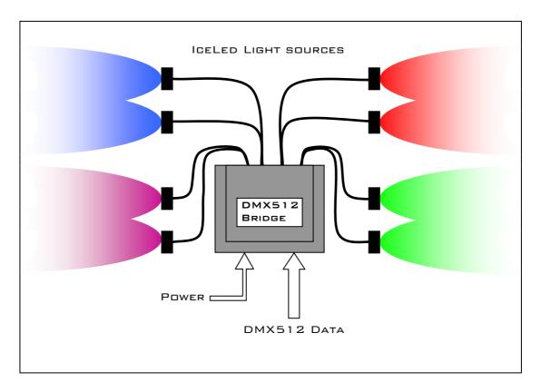
Several ICELED light sources may be connected to each zone in parallel but care must be taken not to exceed the maximum combined current loading of 10 Amps (using a suitably rated power supply). So, for example, if only one zone is to be used then it may be used to supply all 10 Amps. See the user guides for each individual type of light source to be used to find their maximum current ratings.
