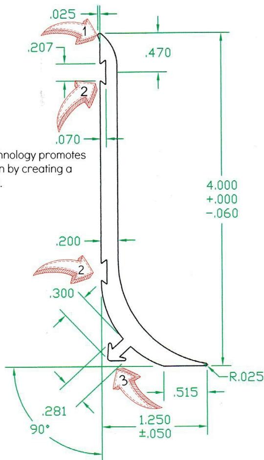
(3) Cove Anchor serves to both anchor the base of the cove to the floor and wall interface, and to lock-out moisture intrusion.
