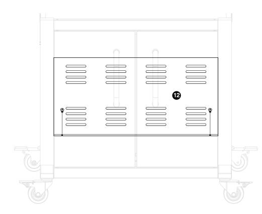
Attach tank block bar to cart using two preattached screws.
