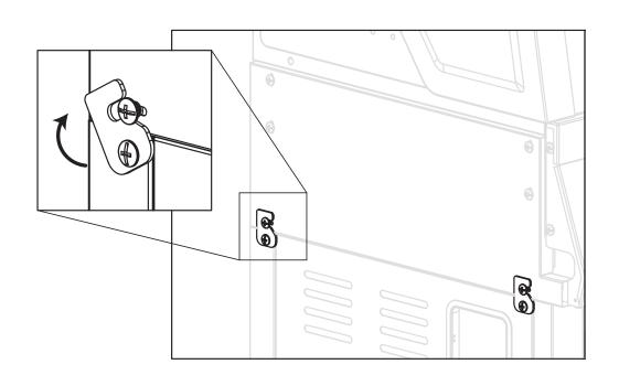
Remove two screws and washers and set aside.
