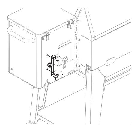
Attach cord wrap using 2 screws just removed.
