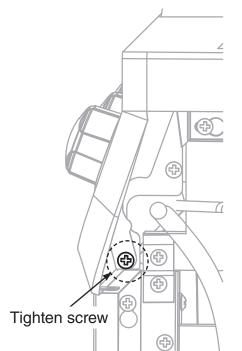
Install screw and tighten (screw was removed in Step 12)
