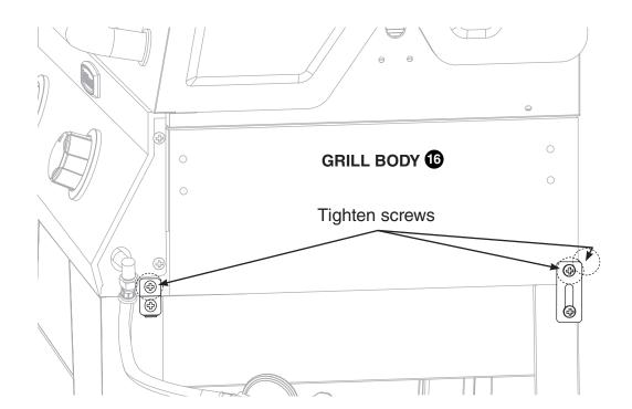
Tighten 3 screws (Removed in Step 16)
