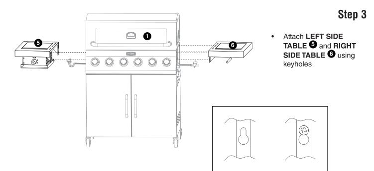
**NOTE:** Before tightening keyhole screws, make sure panels are aligned.
