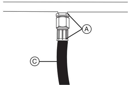
7. Check each place listed (A–D) for growing bubbles which indicates a leak.
