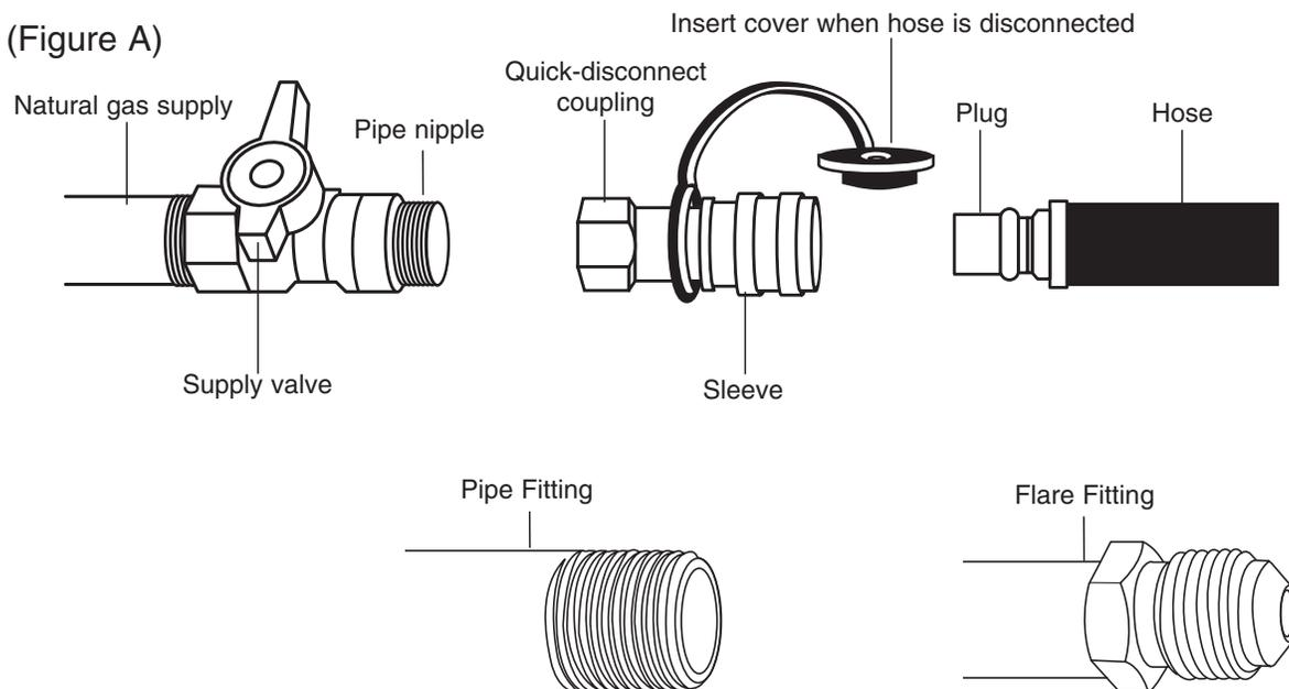
When attaching the quick disconnect to your natural gas supply line, use a pipe fitting, **DO NOT** use a flare fitting.
