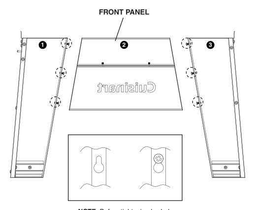
**NOTE:** Before tightening keyhole screws, make sure panels are aligned.
