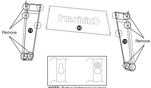
**NOTE:** Before tightening keyhole screws, make sure panels are aligned.
