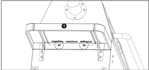
Attach left and right table brackets 7 and 6 to grill body using four preattached bolts.
