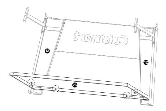
Attach cart base to front legs and using 4 screws removed from Step 1.
