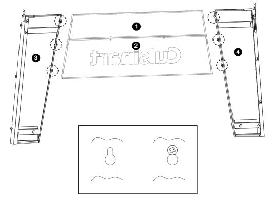
**NOTE:** Before tightening keyhole screws, make sure panels are aligned.
