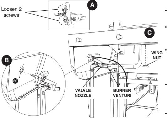
Attach ELECTRODE WIRE to IGNITOR
