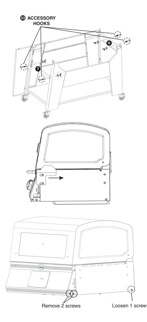
Attach ACCESSORY HOOKS <sup>3</sup> to LEFT SIDE PANEL <sup>3</sup> and CART BRACE <sup>7</sup> with washers and wing nuts
