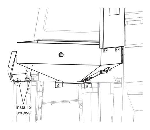
Install PELLET HOPPER LID HANDLE (screws, washers and bezels are pre-installed in handle)
