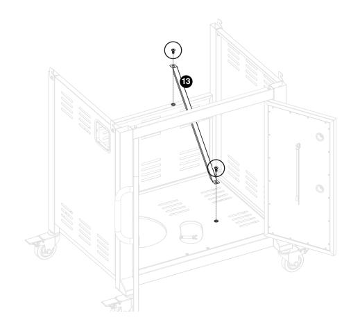
Attach door stopper to cart base using two pre-attached screws.
