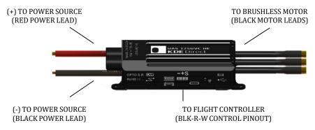
Pay close attention to proper wiring as shown in the diagram above. Ensure the polarity is correct and proper soldering techniques are used when connecting the power source and brushless motor to prevent damaging the ESC.
