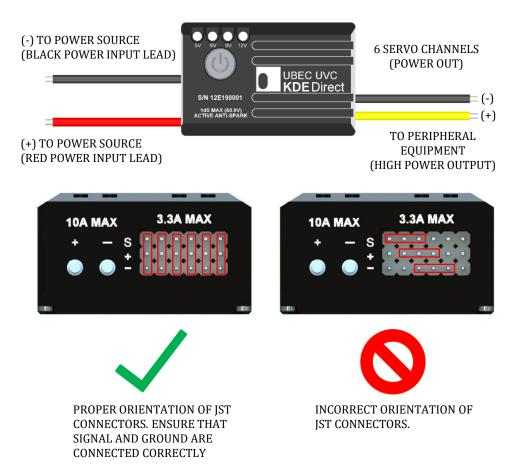
Pay close attention to proper wiring as shown in the diagrams above. Ensure the polarity is correct and proper soldering techniques are used when connecting the power source and peripheral equipment to prevent damaging the UBEC UVC.
