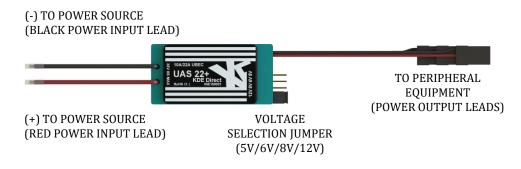
Pay close attention to proper wiring as shown in the diagram above. Ensure the polarity is correct and proper soldering techniques are used when connecting the power source and peripheral equipment to prevent damaging the UBEC. Voltage is selected via the two-pin jumper and can be adjusted before or during operation to control the level of voltage to the peripheral equipment.
