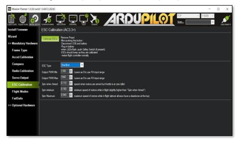
**Note**: program the "ESC Type" to "OneShot" for synchronization of autopilot gyros and ESC control frequencies (400 Hz dynamic).
