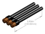
150.0mm exit lead extensions (10 AWG)  $\phi$  6.5mm male bullets pre-soldered
