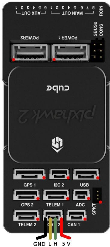
Figure 2: Pixhawk 2.1 (CUBE) CAN bus example.
