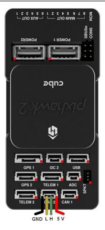
Figure 2: Pixhawk 2.1 (CUBE) CAN bus example.
