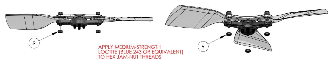
FULLY-TIGHTEN HEX JAM-NUT AGAINST LOWER BASE FOR A MECHANICAL LOCK OF THE PROPELLER BLADE BOLT HARDWARE (SOCKET HEAD SHOULDER CAP SCREWS)
