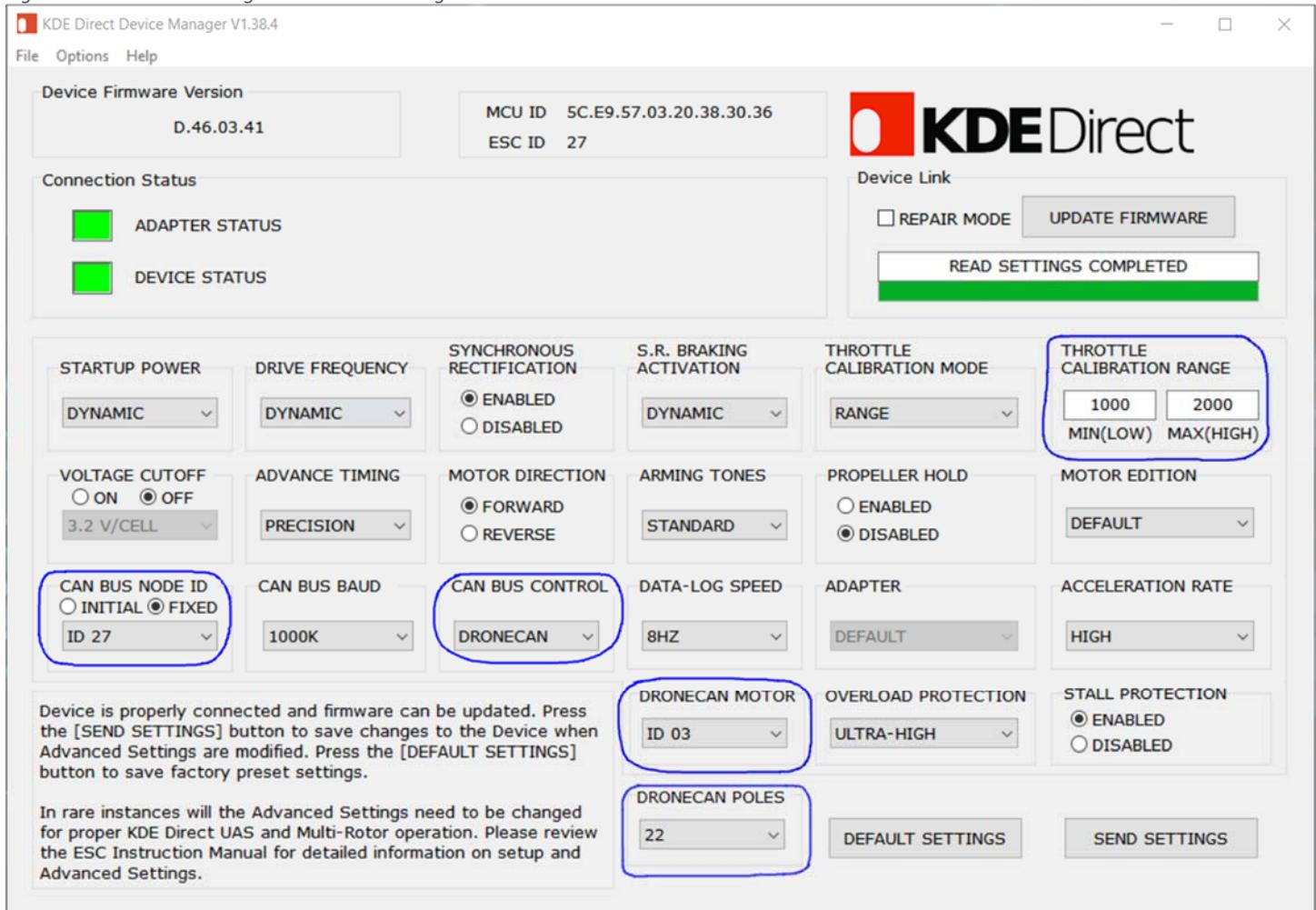
For throttle control to work properly via DRONECAN, first you need to set the CAN\_P1\_DRIVER to 1 and reboot the flight controller (all features that require chunks of memory to initialize are done once at boot). Next, you need to set CAN\_D1\_UC\_ESC\_BM to the number of ESCs you are using in Mission Planner. For example, if you are using a QUAD X frame, then you would select ESC 1, ESC 2, ESC 3, and ESC 4 to enable those motor outputs to be sent.
