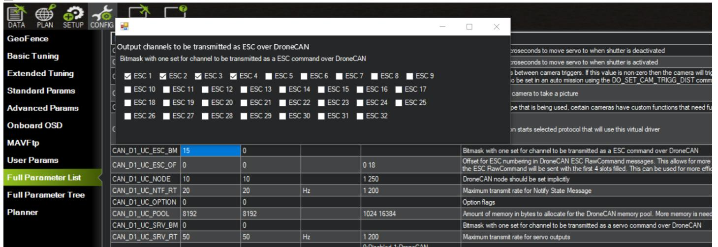
You also need to configure this on each ESC using the KDE Direct Device Manager too. For example, if you're using a QUAD X, the top left motor is ID 3 so the ESC controlling the top left motor needs to have the DRONECAN MOTOR ID set to 03. You will need to set the MOTOR ID for each ESC connected.
