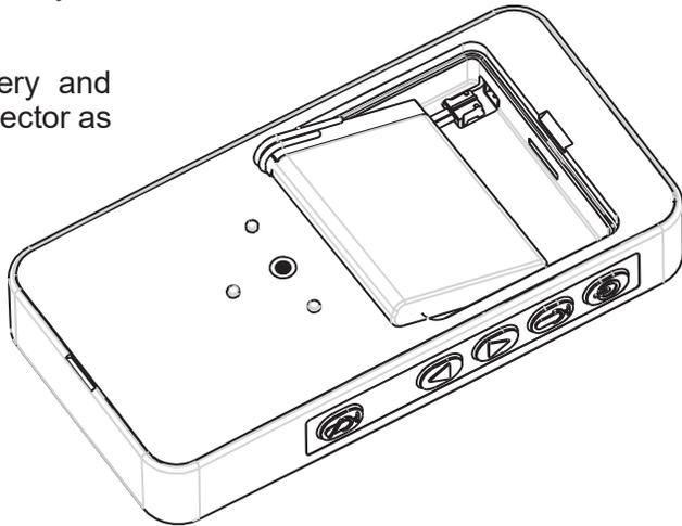
4. Put the battery cover back. Make sure the bump on the battery cover is close to the bottom of the radio.
