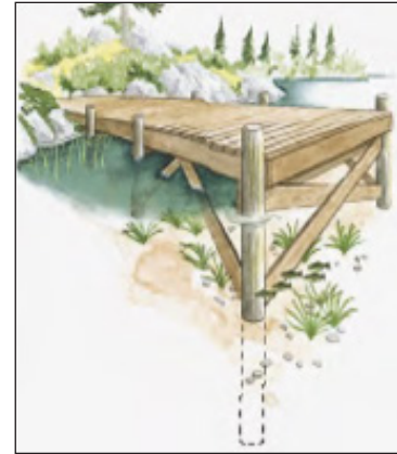
Figure 8: Permanent Post Dock
