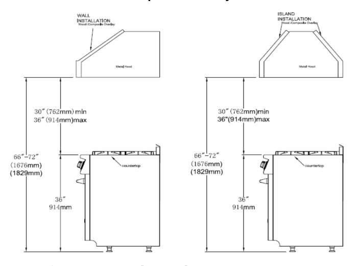
The bottom of the hood should be 30" min. to 36" max above the counter top. This would result in the bottom of the hood being 66" to 72" above the floor. These dimensions provide safe and efficient operation of the hood.
