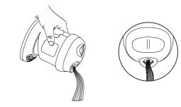
4.When the appliance is not using in a long term (more than several weeks), the water should be completely removed from water tank and steam pipe.
