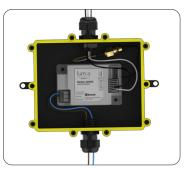
Take in the AC wires from the Mains through a connector (in the box) and connect to the AC Line(Brown) and AC Neutral(Blue) push-in connectors in the device.
