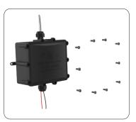
**5** Cover the box with using screws
