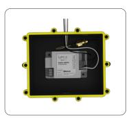
3 Take in the DALI wires from the driver through the connector on the box and connect them to the DALI push-in connectors on the device. Also, take out the wire antenna through the same connector
