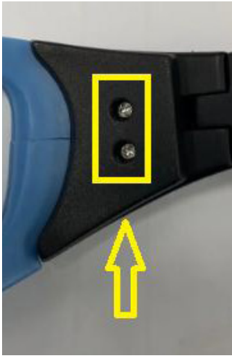
Step 1: Unscrew these two screws.
