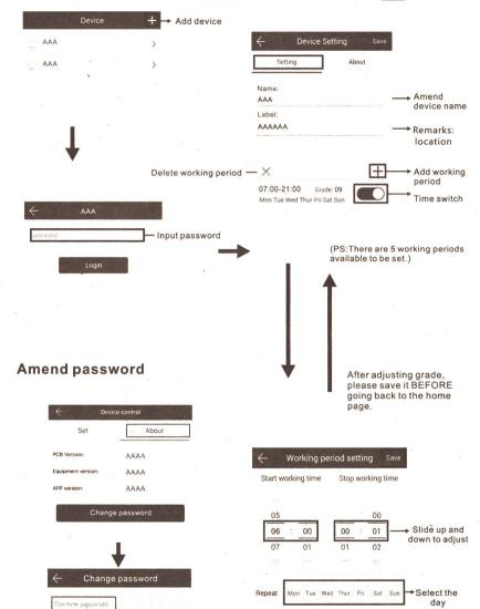
If you forget the password, please press the reset button to restore the factory settings. The factory settings password is 8888.
