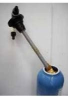
Insert the check valve riser into the full container and screw the lid on.
