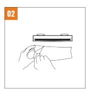
Expose the adhesive on the disposable trap.
