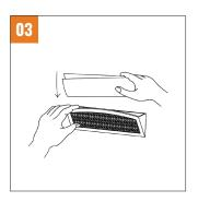
Place the disposable trap inside the plastic housing.
