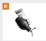
Invert the bulb and shake to get dust into the rod.
