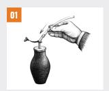
Secure the flexible vinyl tubing onto the brass tip.
