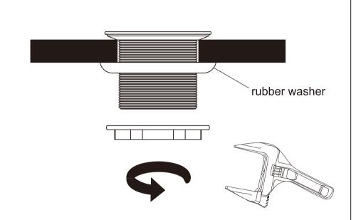
2. Put the thread pipe through the bath hole. Fit the rubber washer and tighten up the nut on thread pipe by screw driver.
