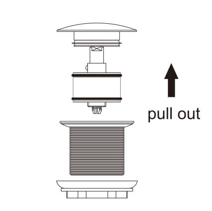
1. Disassemble pop -up waste by pulling out the cap.
