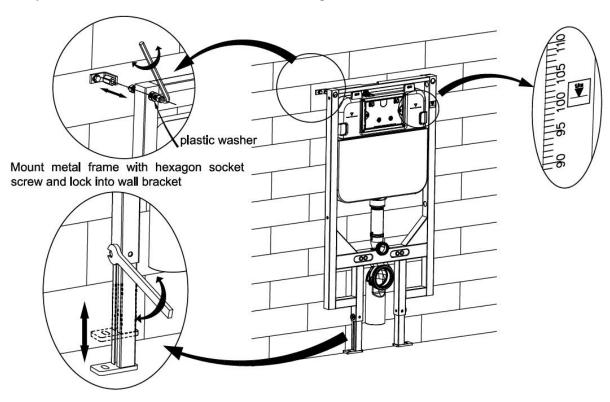
5. Adjustment and fixation of mounting frame
