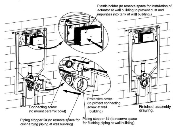
7. Wall thickness range 20-60mm (from frame outside surface to finished wall)
