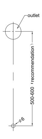
1.Drill a  $\phi$ 6mm hole at the downwards outlet vertical downward position in the recommended range.
