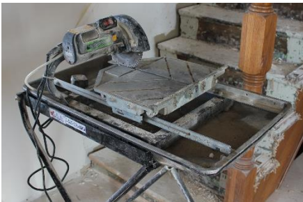
Above: Wet saw used for thin stone veneer.
