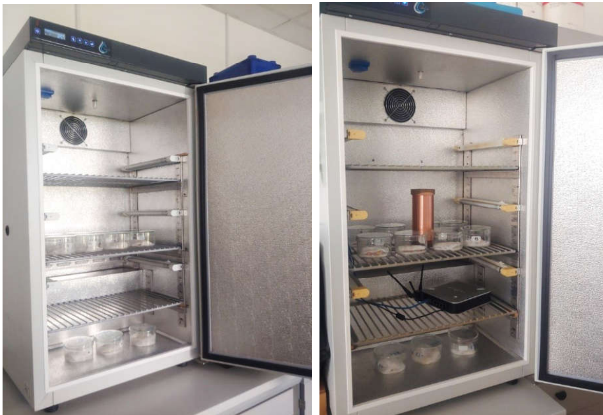
Figure 1: Growth chambers and arrangement of glass containers with beans. Left: control experiment, right: experiment where beans were exposed to Wi-Fi and Qi-Shield.
