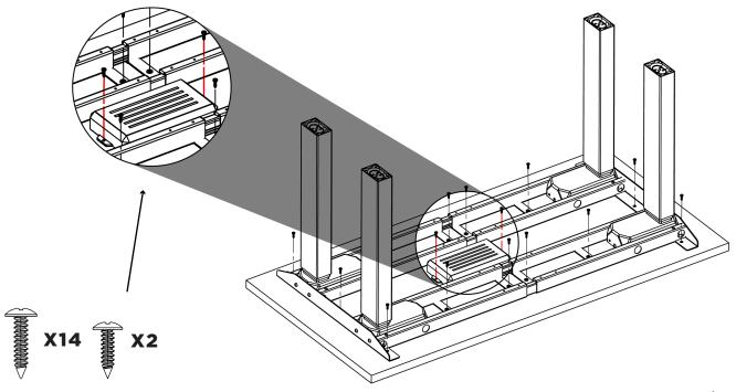
**IMPORTANT:** Do not tighten machine screws fully until the end of each step to allow for proper centering.
