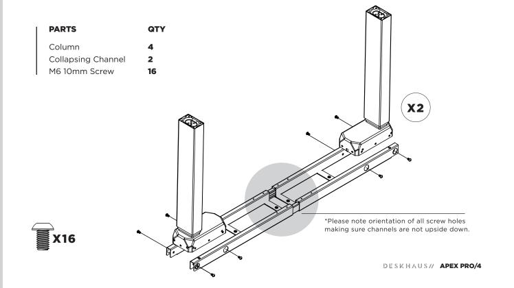
IMPORTANT: Do not tighten machine screws fully until the end of each step to allow for proper centering.
