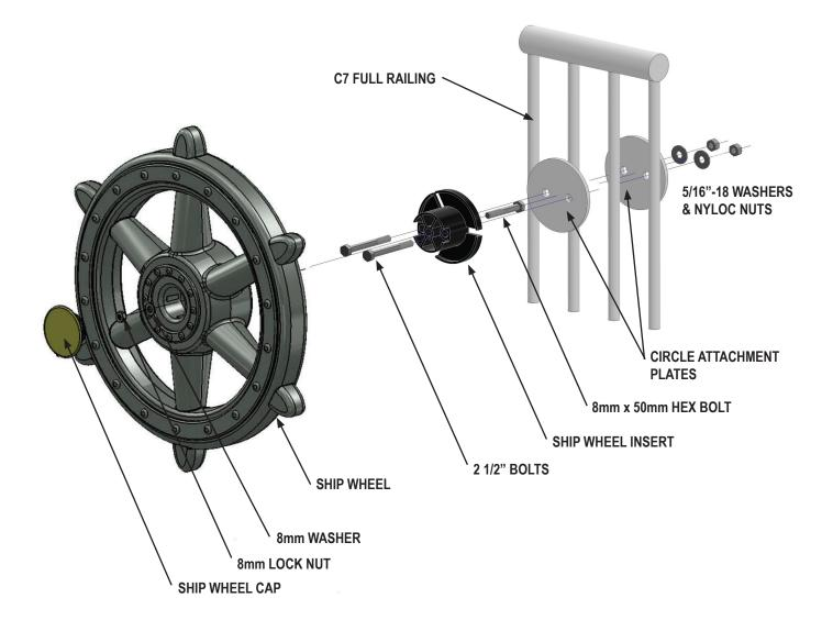
STEP 1: Place the 8mm x 50mm L hex bolt into the hex recess in the back side of the Ship Wheel Insert.
