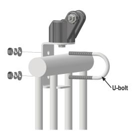
**STEP 4**: Slide the spotlight onto the plastic bracket and bolt together using the bolt, washer, and nyloc nut provided.
