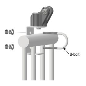
**STEP 4**: Slide the telescope onto the plastic bracket and bolt together using the bolt, washer, and nyloc nut provided.
