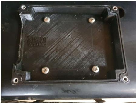
Fit upper section of the control box to the lower mount. Ensure the seal is in place during assembly.
