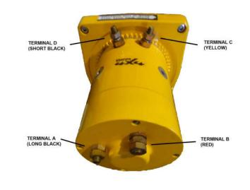
Note: When testing, if your winch hand controller is opposite to the labels, eg, 'Winch in' functions as 'Winch out', connections at terminals C and D can be swapped.
