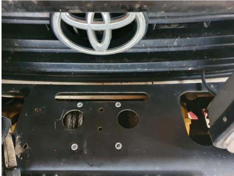
Add a silicon sealant at all holes to limit corrosion at the mount and also stop water ingress into the control box.
