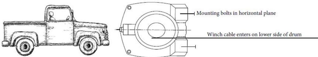
Mounting your winch with the bolts in the horizontal plane with the bolt heads facing the vehicle in front of you is the strongest mounting arrangement as it takes much of the winching force off the mounting bolts and winch foot mount. The rope/cable should enter the drum on the lower side of the drum in keeping with the direction labels on the winch. Ensure your mount is rated for the force that can be applied.
