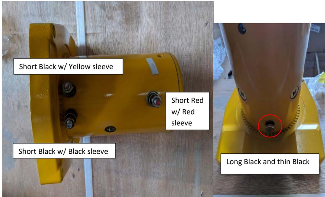
**Take care, failure to correctly connect the cables may result in motor damage.**
