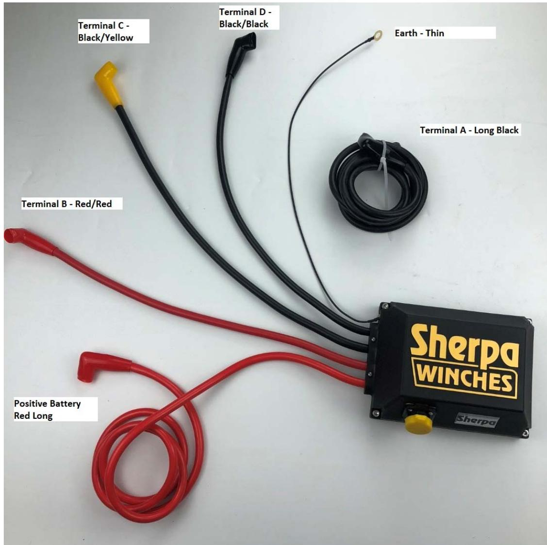
Note: Swapping cable connections at terminals C and D on the motor will reverse the winch operating direction relative to the remote controller buttons.
