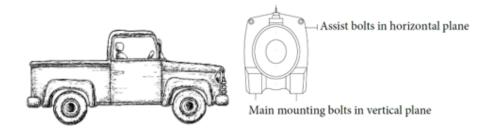
Unbalance in forces during winching can test the design limits of the winch mount and bolts. To limit the potential for a bolt shear failure, note the following;
