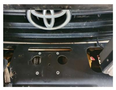
Add a silicon sealant at all holes to limit corrosion at the mount and also stop water ingress into the control box.
