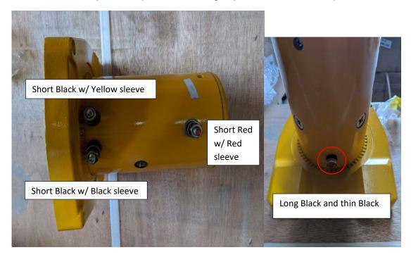
Take care, failure to correctly connect the cables may result in motor damage.
