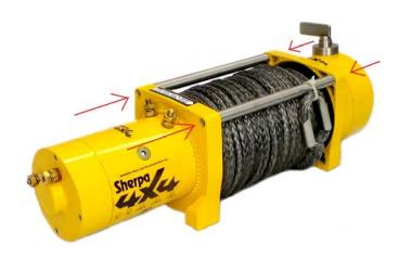
Winches are mounted in a high vibration environment. It is highly recommended both liquid thread locker and spring washers are used on all connections. All connections should be checked for tightness after 1,000km of travel.
