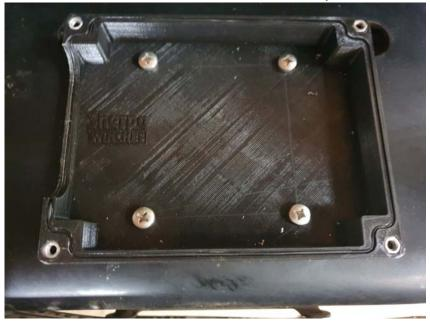
Fit upper section of the control box to the lower mount. Ensure the o-ring seal is in place during assembly.
