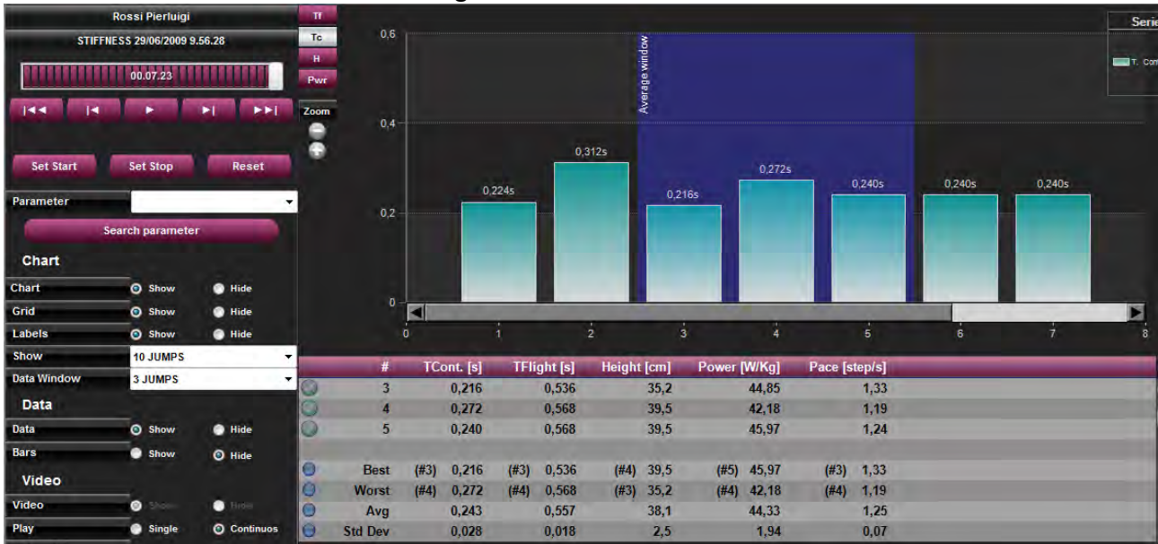
Figure 63 – Display 10 events at a time and take 3 of them into consideration (blue window)
