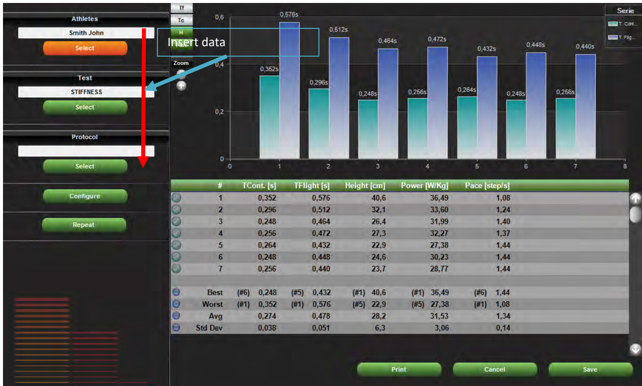
Figure 34 -ExecuteTo perform a trial it is advisable (but not obligatory) to follow the direction of the operations indicated by the red arrow at least the first time you enter this section.
