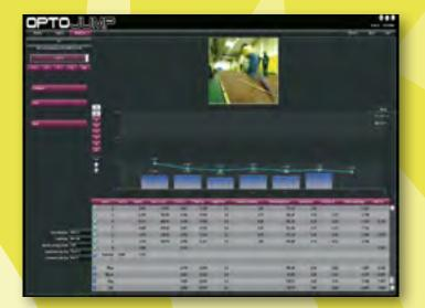
Real time viewing of the data acquired during performance of a test, with video analysis, graphs and numerical data of the specific parameters. The data saved can be retrieved and analyzed in any moment.
