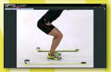
Processing of a video still image acquired during a test, with the possibility of graphical interventions and measurements of angles and legths.
