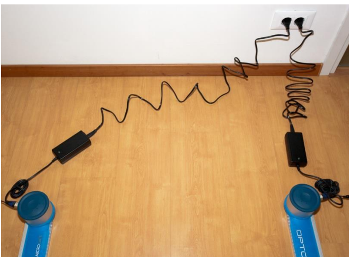
Figure 25- Two power supplies for multiple-meter systems
