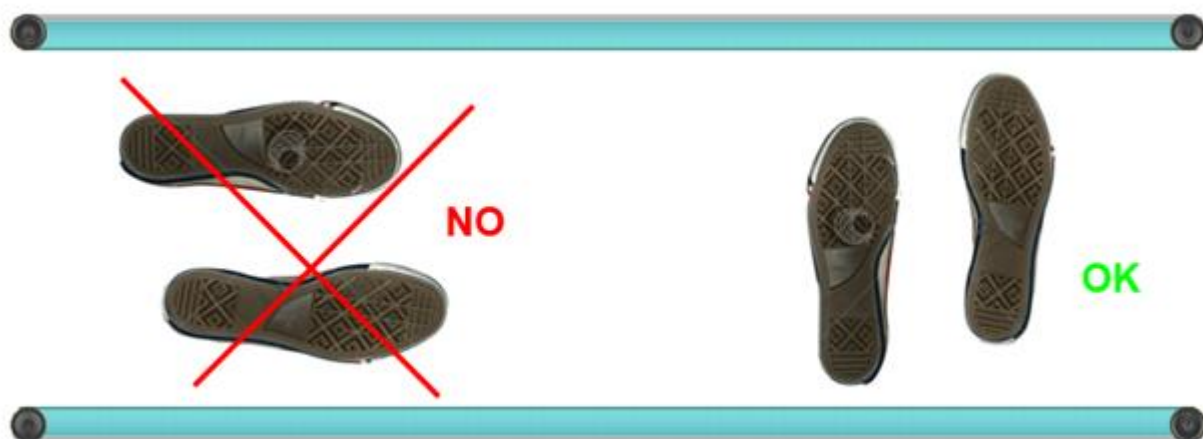
Figure 53 – Correct execution of a Tapping Test
