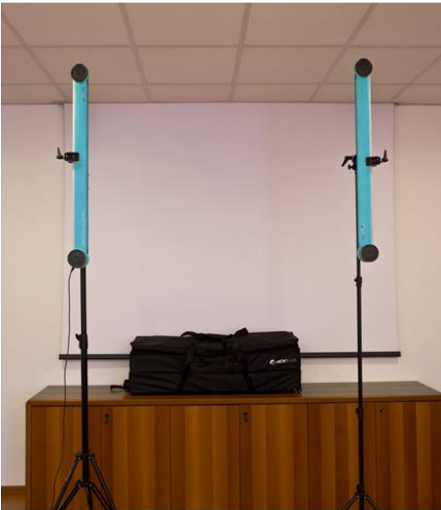
Figure 144 - VERTEC LIKE test setup
