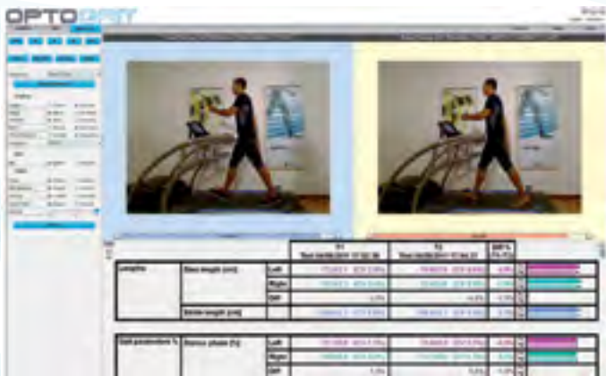
Comparing two tests with compared Gait Report and videos (T1 = test with shoes, T2 = barefoot test)
